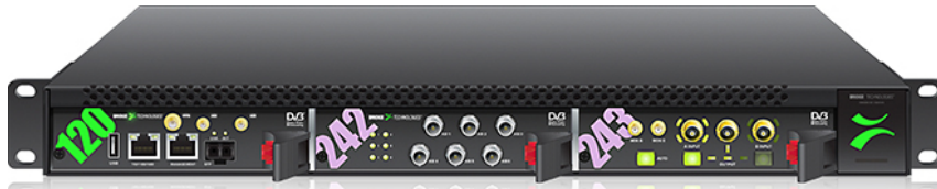
Figure - Pictured is a complete VB243 system with a VB120 controller, a VB242 ASI input blade and a VB243 ASI 2:1 switch blade housed in a 1RU Redundant AC powered chassis. Not shown are the two factory fitted connecting cables between port 1 and 2 on VB242 and the VB243 switching module. The power consumption of this configuration is a modest 25W giving additional savings in operational costs.
