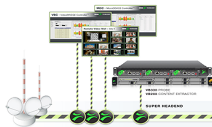
Figure - VB288 is typically deployed in the master head-end prior to encryption.
